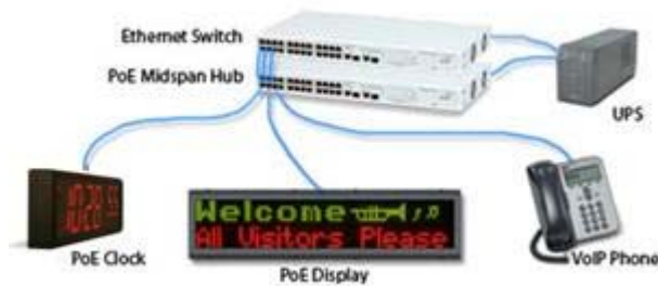
Example of common PoE configuration
