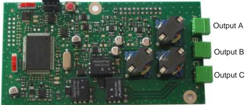
This option board does not require any software programming (by default the time is the local time defined in the Sigma and the line is stopped). Only the time zone differential and the state of the line (On / Off) is to be defined in the “Time outputs” technician menu (see page 27).
