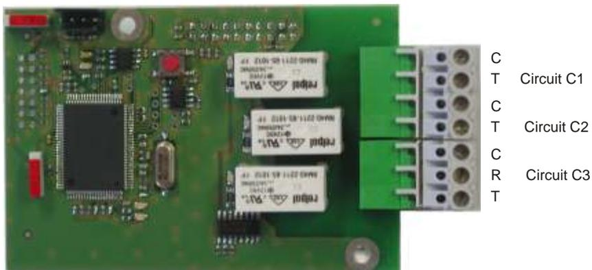
This option board does not require any software programming. It allows 3 relays to be added. See the technician menu (circuit setting programming) on page 30.
